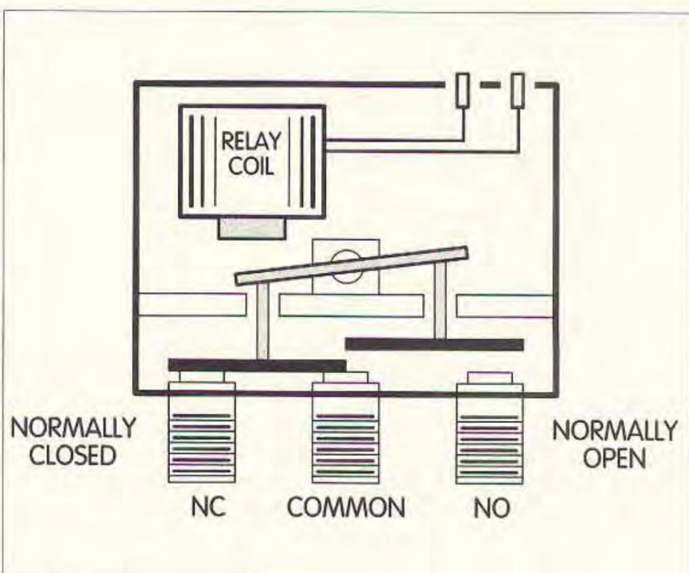
*Fig. 1. Microwave switch internal construction. Note balanced actuator arm that pushes bar contact from grounded out-of-circuit position to contact from one side of switch to center contact. Left or right side of switch operation identical. Typical frequency of operation from VHF to 24 GHz. Size of switch decreases to reflect increases in frequency.*
