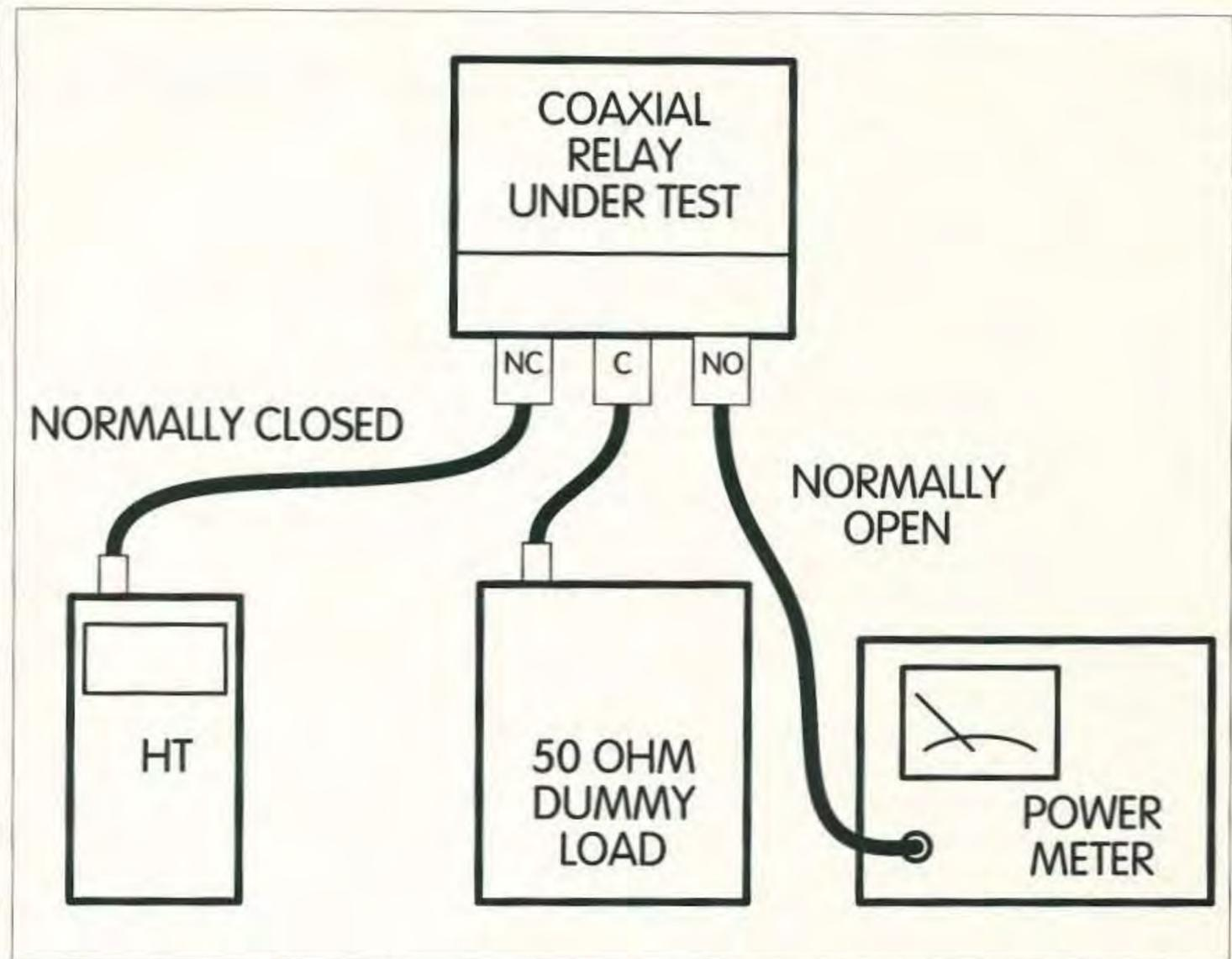
**Fig. 2.** Test setup to measure isolation between switch ports. Signal generator (transmitter) places power through contacts of switch. Power measurement made at open switch contact to verify isolation of switch. Isolation should be better than 50 dB for a good switch.
